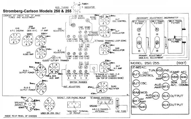
Terminal Layout for Voltage Measurement Chart and Location of the Various Aligning Adjustments.
