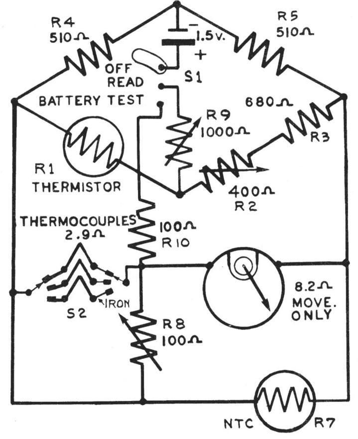
FIGURE 3. SCHEMATIC DIAGRAM FOR SIMPSON THERM-O-METERS, MODELS 388 AND 388-3L
