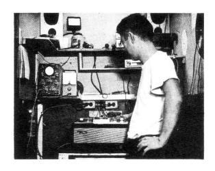
Here in this insulated, sound-proof booth, protected completely from factory noise, each Seabreeze unit is carefully inspected and tested immediately prior to packing. In addition, other units are periodically given gruelling "torture tests" to make sure they will give dependable service to Seabreeze customers.
