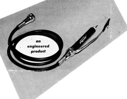
The new PRECISE RF PROBE, although one of the lowest priced in the electronics field, consists of a time tested circuit firmly housed in a specially constructed non-porous case. It uses a GERMANIUM CRYSTAL rectifier for measurements up through 250 megacycles. The probe handle is terminated in an amphenol connector while the other end of the shielded cable may be obtained with either an amphenol, phone plug or phone tip type of fitting, at no extra charge.
