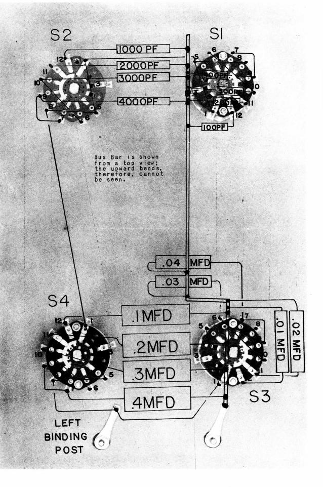
You have now completed the wiring of your Model 478. Check all soldering carefully, making certain each connection is soldered and there is no rosin between them. You may, if necessary, clean the contacts with carbon-tetrachloride. With each switch in its maximum counter-clockwise position (as observed from the front of the panel), place small pointer knobs on shafts with indicator at zero mark. Secure panel to cabinet with four screws.
