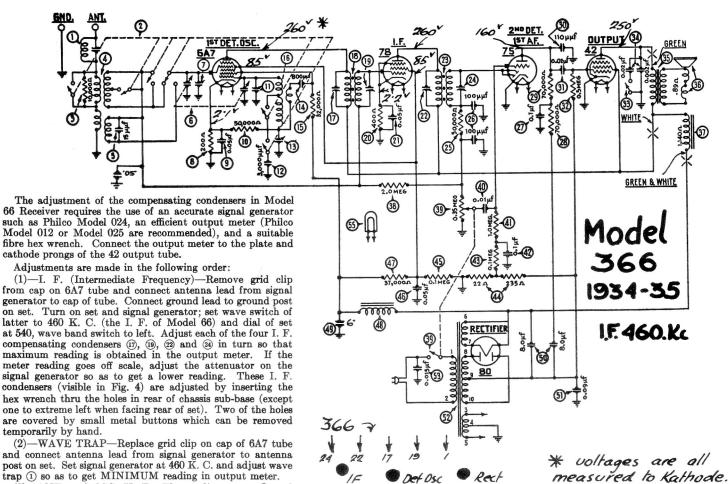
(2)-WAVE TRAP-Replace grid clip on cap of 6A7 tube and connect antenna lead from signal generator to antenna post on set. Set signal generator at 460 K. C. and adjust wave trap 1 so as to get MINIMUM reading in output meter.
