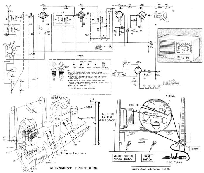
CAUTION: One side of the line is connected to chassis; DO NOT GROUND CHASSIS.
