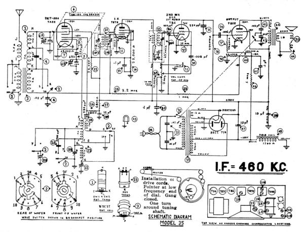
NOTE: Voltages shown on schematic diagram were measured with a 1000 ohm per volt meter such as Philco Model 026 or 028. Line voltage was 115 volts, volume control maximum, tone control high, tuning condenser closed and wave switch in "B'DC'ST" position.
