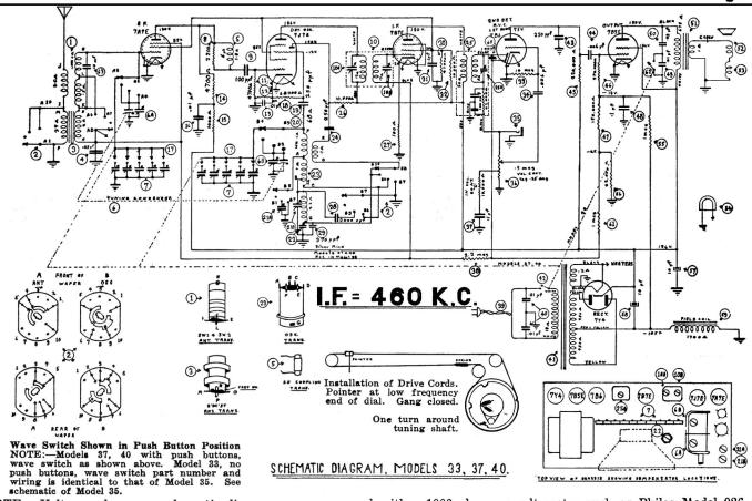
NOTE: Voltages shown on schematic diagram were measured with a 1000 ohm per volt meter such as Philco Model 026 or 028. Line voltage was 115 volts, volume control maximum, tone control high, tuning condenser closed and wave switch in "B'DC'ST" position.
