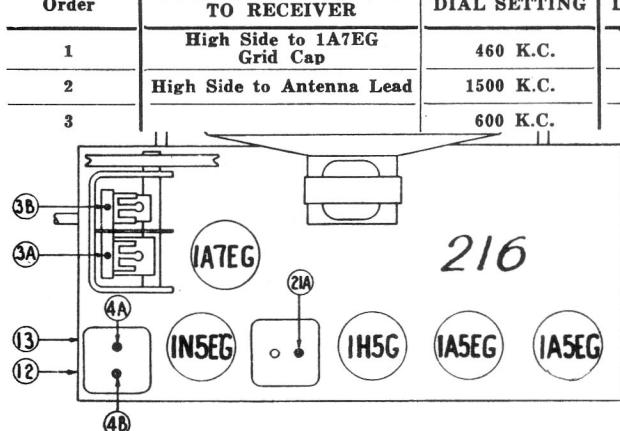
**NOTE A**—When adjusting the I.F. padders the high side of the signal generator is connected through a .1 mfd. condenser to the cap of the 1A7EG tube. The ground side of the signal generator is connected to the ground lead of the receiver.
