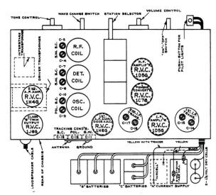
In order to properly realign this receiver the radiotrician should have available an output meter and a well attenuated test oscillator capable of giving the following frequency fundamentals:-
