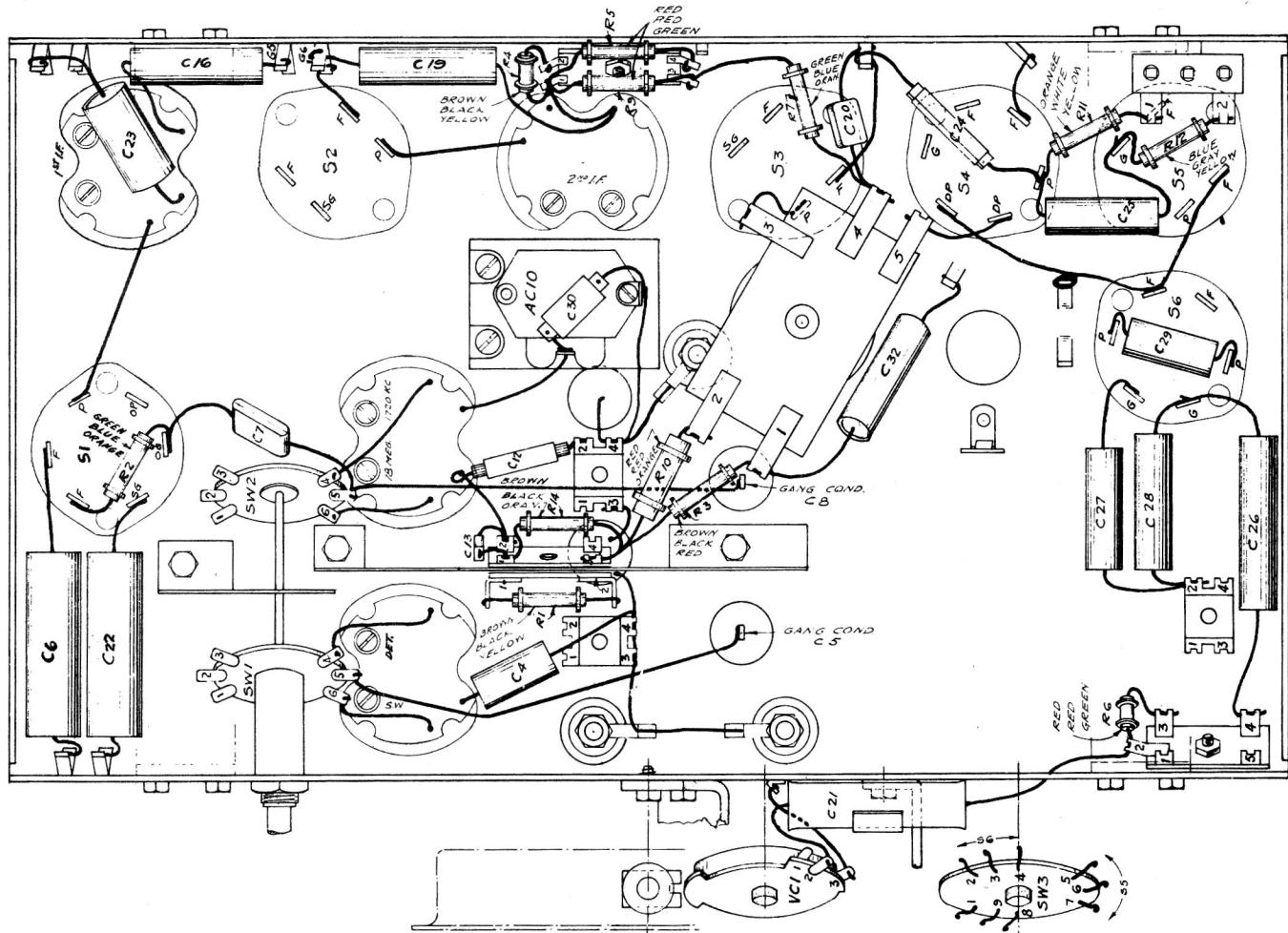
*Figure 2—Chassis Wiring Diagram*
