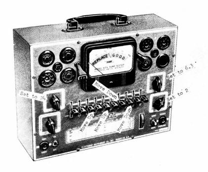
If more than one listing is given on the roll chart (6SQ7, 6J6, etc.) it is because the tube under test is multipurpose. The procedure is to test the first row of figures, then reset and test the second, third, etc. If any test shows bad, the tube is defective.
