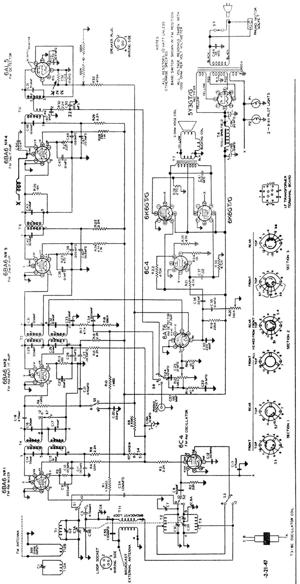
**Power Supply**.....105 to 125 volts, AC, 60 cycles; Chassis only 90 watts. With phone operation 115 watts.
