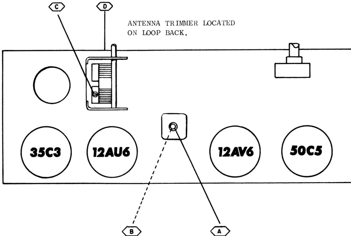
**ADJUSTMENT "A" ACCESSIBLE FROM BOTTOM OF BOARD**
