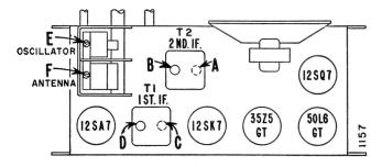
Adjustments A and C are made from underside of chassis.
