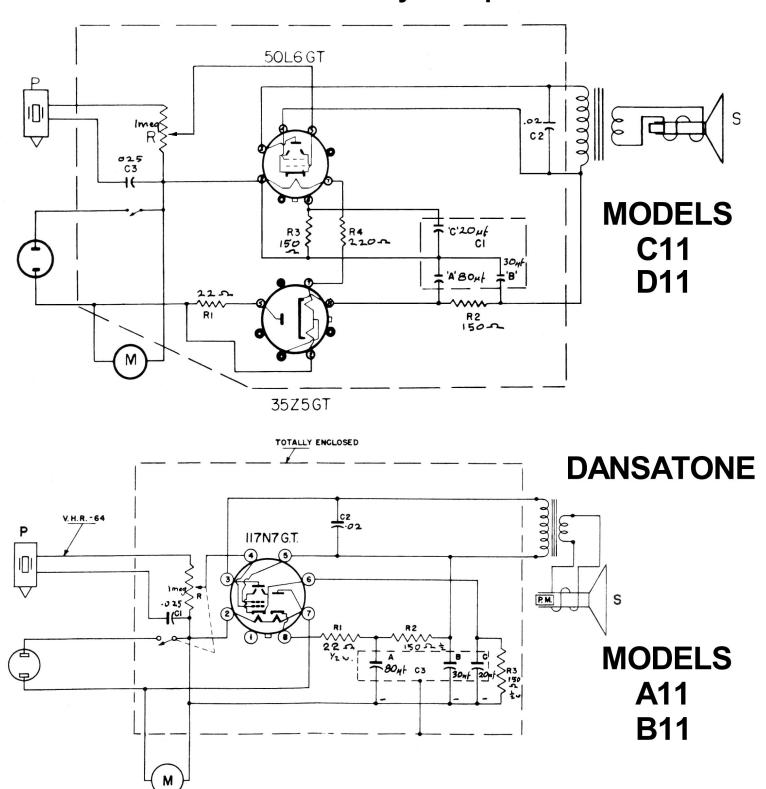
If Dansatone fails to operate, check the power cord to determine that proper contact has been made. If satisfactory, remove screws holding the panel and remove the unit. A visual inspection may only be necessary, however, if all is in order, remove the Volume Control Knob, Hex Nut and Mounting Screw. This permits the Amplifier to be removed and all component parts may be checked by aid of the schematic.
